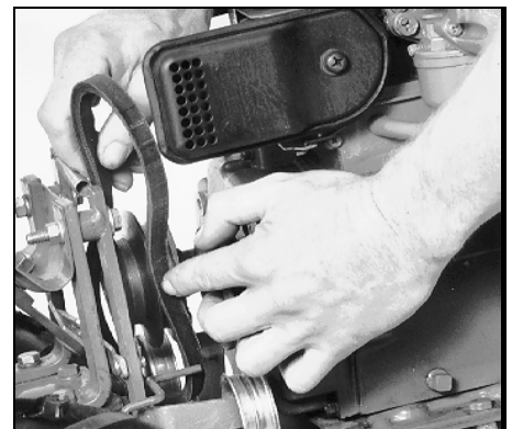
Figure 5-17: Install forward drive belt over rear of engine forward pulley and bring lower half of belt down and in front of transmission pulley.
